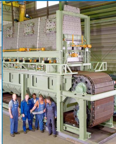
Curing oven for glass wool pipes (special Münstermann construction)
